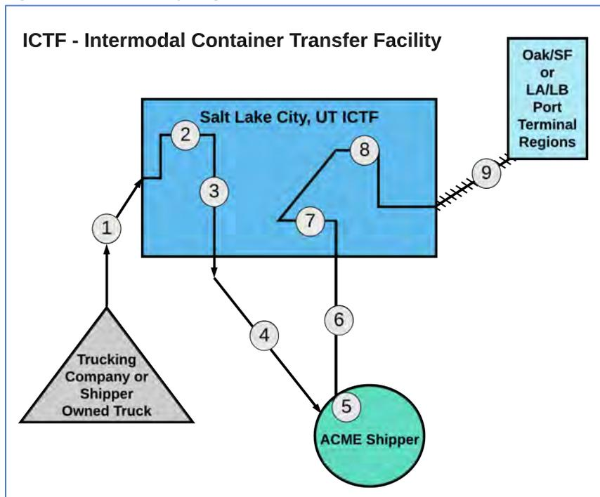
Exhibit 1 demonstrates the nine steps involved to accommodate an export container loaded via an ITCF operation. The ITCF process is driven by the need for cargo loading at the shipper location into special equipment necessary for rail transportation.
